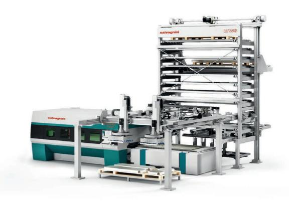
In the laser world, automation is playing an increasingly key role: on the one hand, cutting speeds risk turning loading and unloading into hazardous bottlenecks, and on the other hand, automation can help to reduce the impact of labor costs. **The loading/unloading and sorting connections satisfy all automation requirements**: from stand-alone operation, to integration in flexible cells or in automatic lights-out factories.
